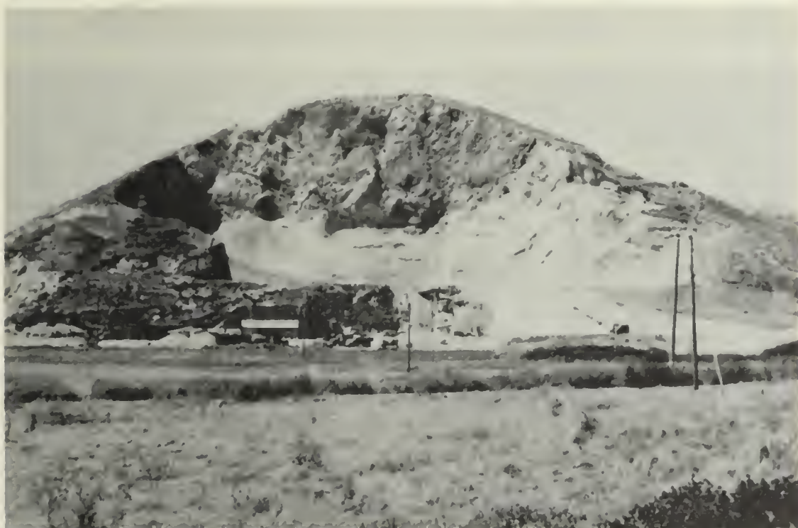
B, VIEW WEST TOWARD ROCKAWAY QUARRY Rockaway Beach, San Mateo County. Quarry is in Jurassic (?) Calera limestone, which is used for road construction. Fenelon F. Davis, photography, 1949.
